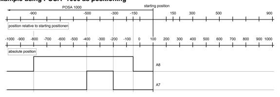
Cam controller with compensation for switching delays
